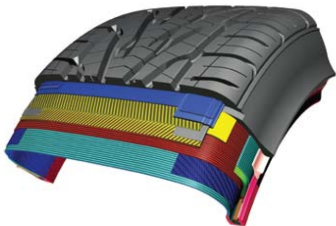
Figure 1: This image shows the complex layering of materials that compose a Goodyear tire. All of these components are simultaneously considered during the modeling and simulation process.
