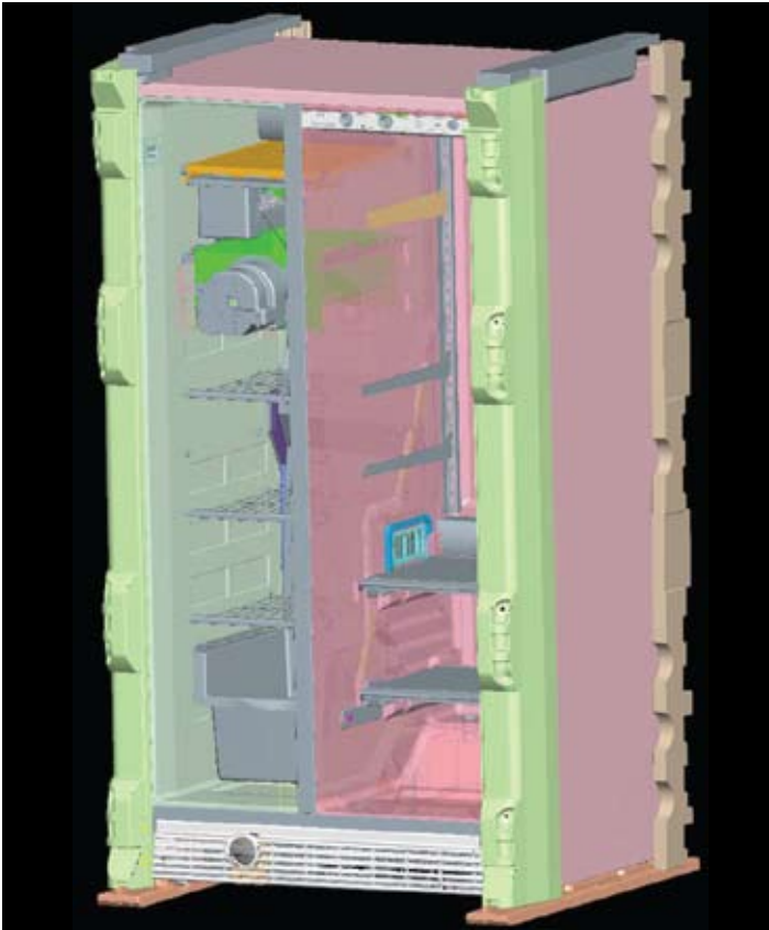
With HPC, Whirlpool is able to model, simulate and analyze (e.g., CFD, FEA, etc.) their products as complete systems, as in this image showing a refrigerator master assembly, including packaging material for transportation.
