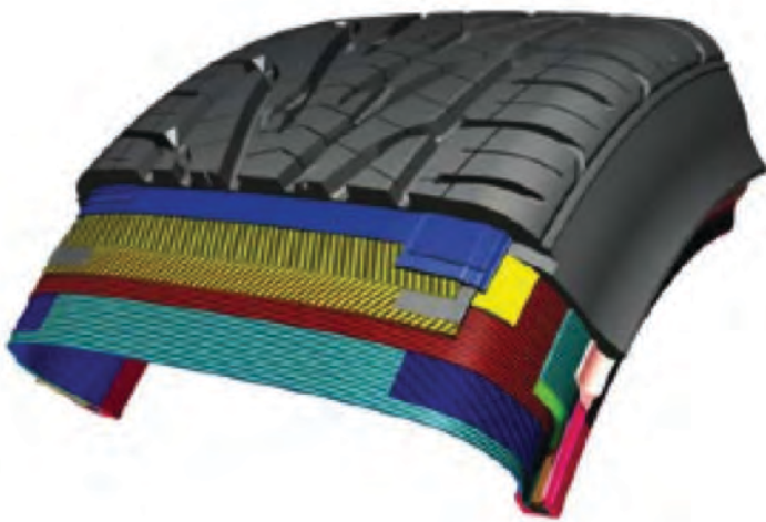
Figure 2. Complex Layering of Material Used in a Goodyear Tire
