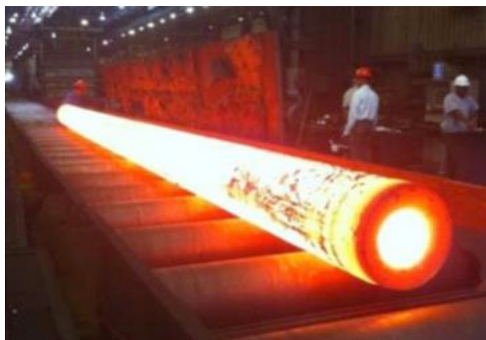
Figure 1: Extrusion of Inconel 740H Pipe at Wyman Gordon plant
