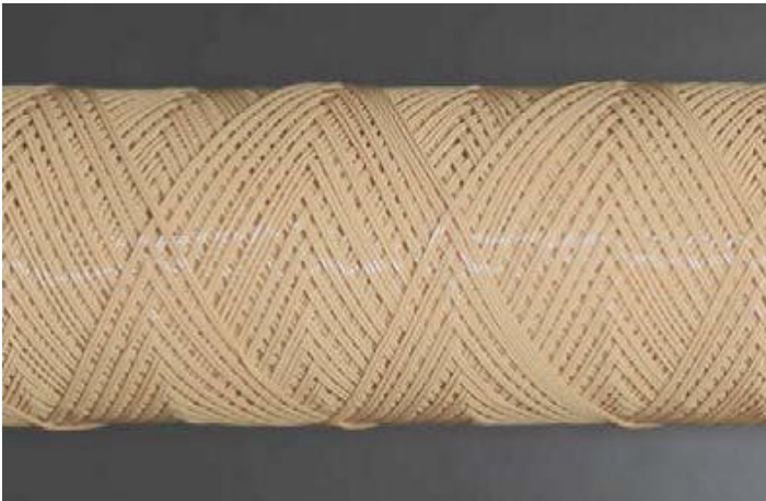
Figure 2: PEEK Hollow fiber membrane contactor developed to increase the efficiency of carbon capture from power plant flue gas
