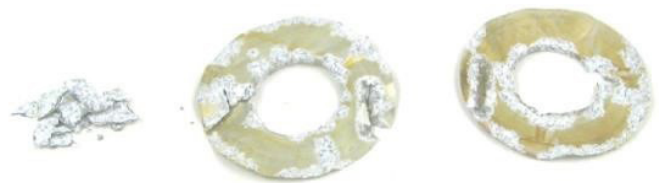
Figure 3: Aluminum fins from a geothermal power plant subjected to 24,000 cycles of exposure to briny conditions with: no protective coating (left), nano-coating with a low level of Cerium Oxide (middle), and a nano coating with a higher concentration of Cerium Oxide (right).
